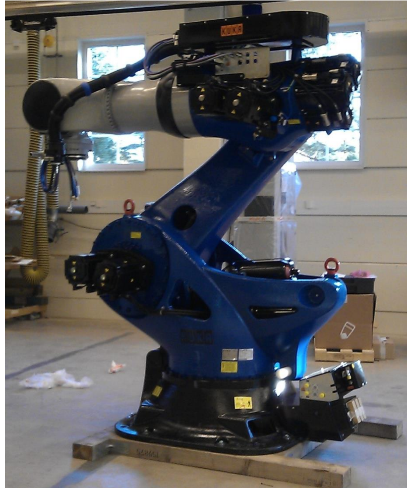
Robot (Backfilling of deposition tunnels)
