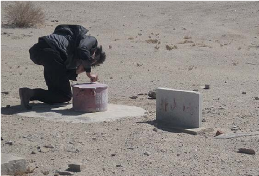
Fig. 6 – Exploring the site for a high level waste deposit: a scientist is checking a drill hole in Beishan, Gansu Province [3]
